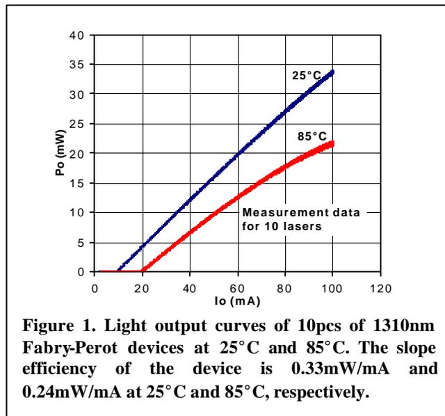
**Figure 1. Light output curves of 10pcs of 1310nm Fabry-Perot devices at 25°C and 85°C. The slope efficiency of the device is 0.33mW/mA and 0.24mW/mA at 25°C and 85°C, respectively.**
