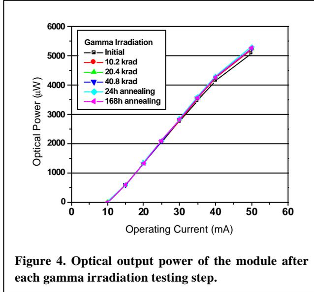
Figure 4. Optical output power of the module after each gamma irradiation testing step.
