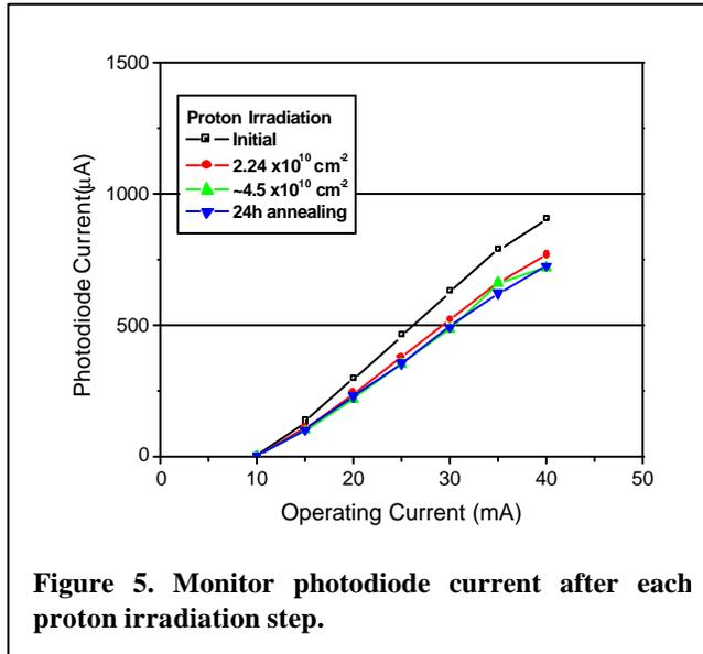
Figure 5. Monitor photodiode current after each proton irradiation step.
