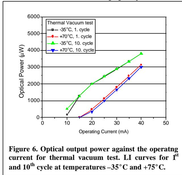
**Figure 6. Optical output power against the operating current for thermal vacuum test. LI curves for 1<sup>st</sup> and 10<sup>th</sup> cycle at temperatures –35°C and +75°C.**
