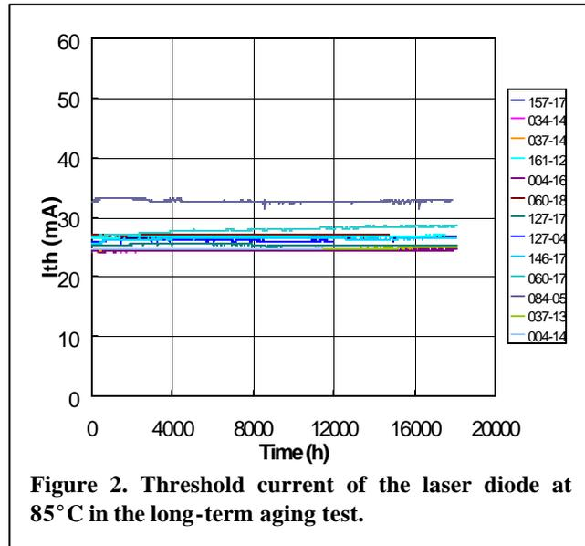
Figure 2. Threshold current of the laser diode at  $85^{\circ}\text{C}$  in the long-term aging test.
