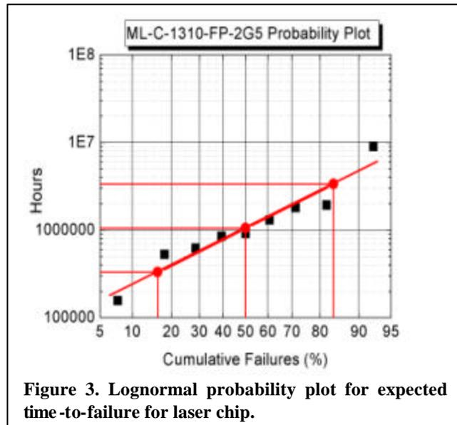
Figure 3. Lognormal probability plot for expected time-to-failure for laser chip.
